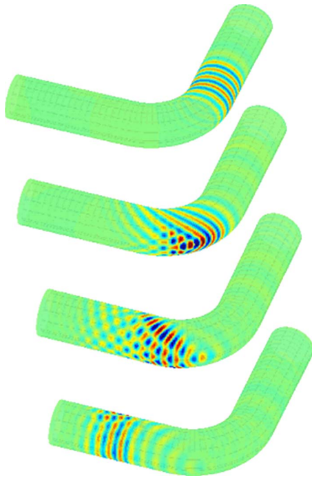
FIG. 13. (Color online) A 50-kHz guided elastic wave propagates through a 90° pipe bend. The guided waves naturally focus at the back of the bend.
