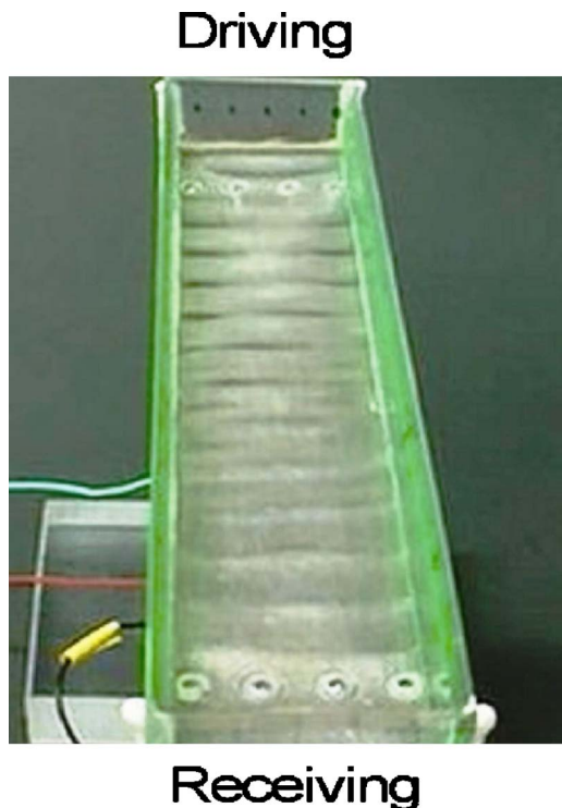
FIG. 11. (Color online) The undulating pattern formed by the vibrating plate.
